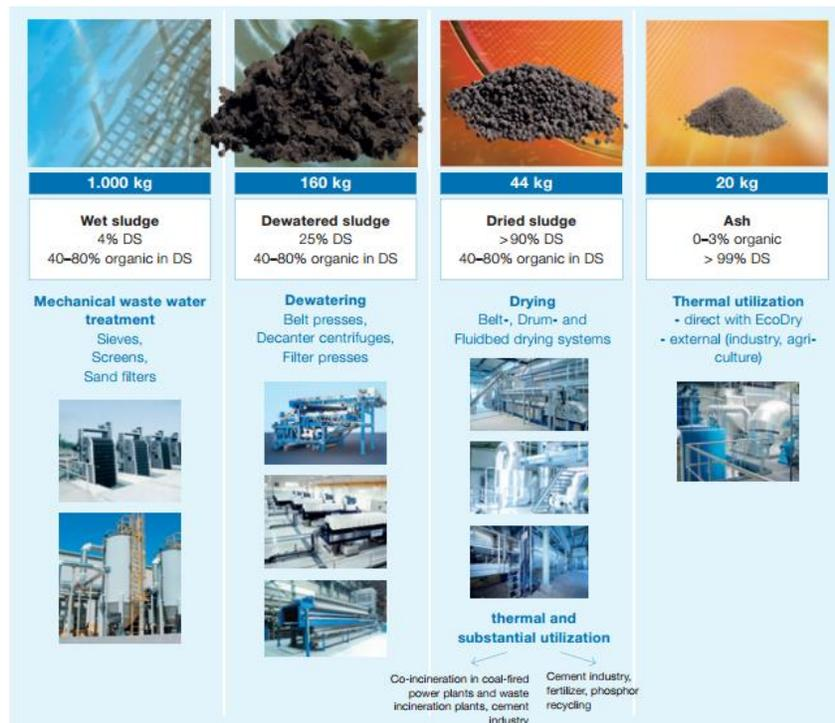
The below infographic illustrates the end uses possible from the drying technologies offered by Andritz:
